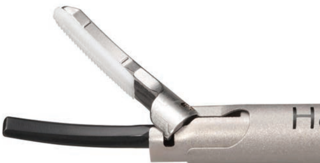
Figure 14-19. Ultrasonic shear. When closed vibration of black (active blade) against white (passive blade) cuts and cauterizes intervening tissue.
